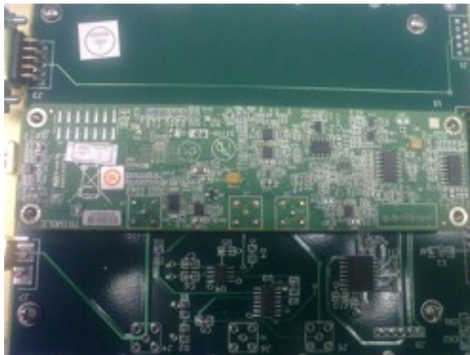
Picture 7: Remove the GPS board mounting screws
