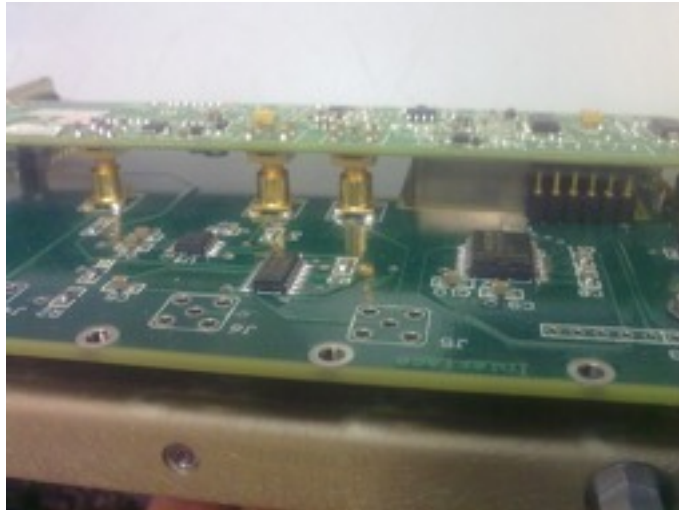
Picture 8: Align the mini GPS board connectors to the GPS module connectors.
