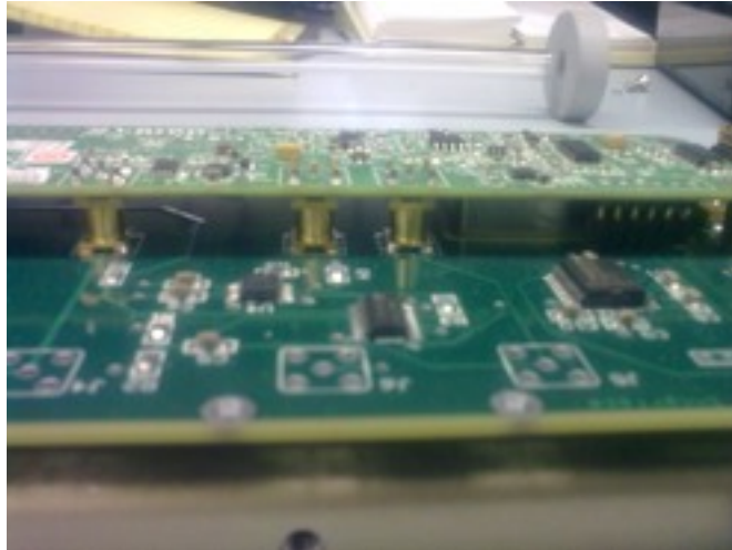
Picture 6: mini GPS board snapped onto the GPS module
